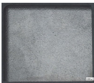
As-built, heat treated and abrasively blasted
