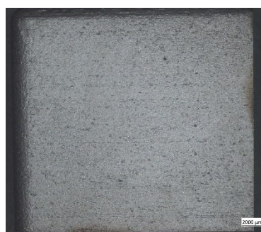
As-built, heat treated and pickled
